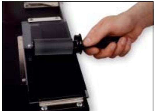
An operator uses the No. ATP1001 to apply ink to an inking slab.
