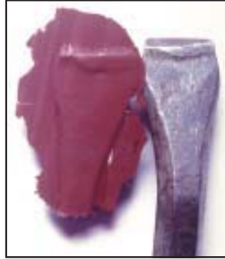
Mikrosil™ used to cast a door jam where a pry bar was used to gain entry.
