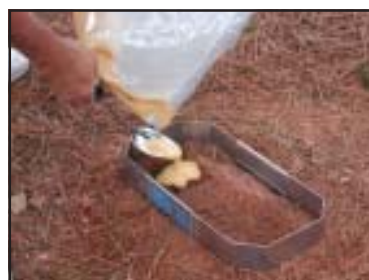
STEP 4: Pour mixed casting material into impression*. (* Optional accessories shown.)
