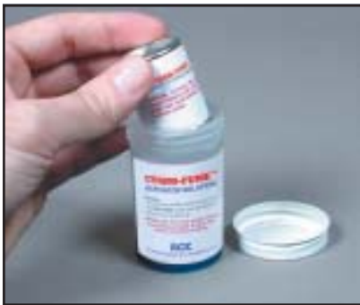
Step 1. Place the activator canister (hole side down) into the jar containing activator solution.
